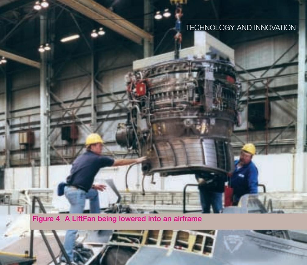
Figure 4 A LiftFan being lowered into an airframe
