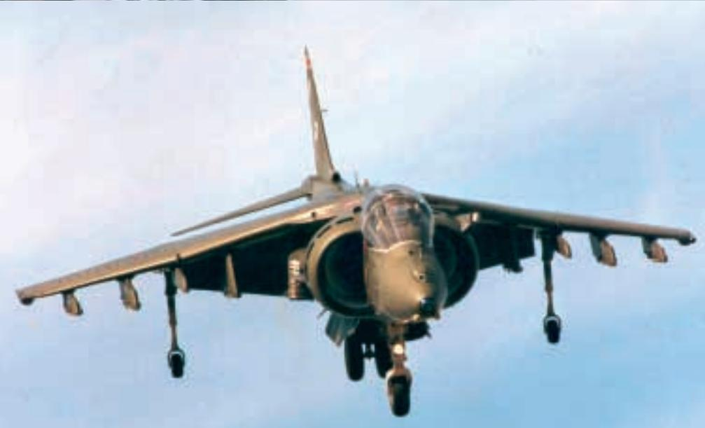
Figure 5 The Harrier uses vectored thrust for STOVL
