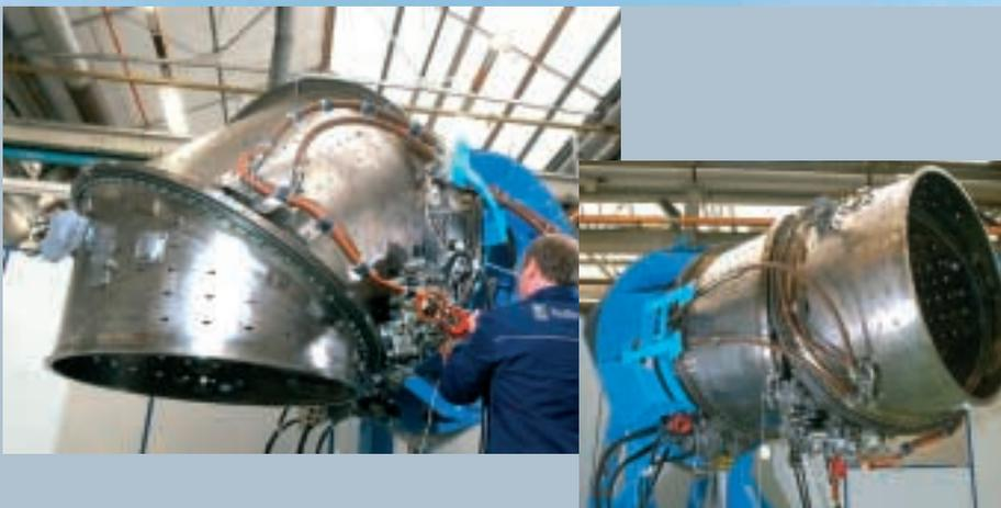
Figure 6 The 3 Bearing Swivel Module, a key module of the LiftSystem, can turn through 90 degrees in just over 2 seconds
