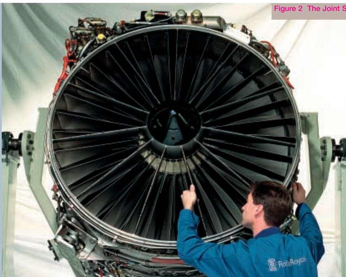
Figure 2 The Joint Strike Fighter F-35 LiftFan
