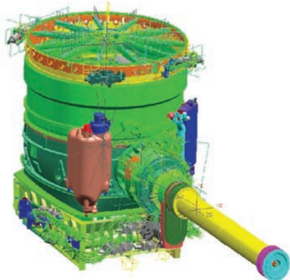
Computer simulation of LiftFan with gearbox, clutch and drive shaft. The gearbox takes 29,000hp from the main engine and transfers it through a right angle to drive the LiftFan rotor © Rolls-Royce
