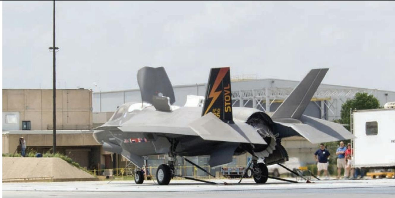
BF-1 pit testing Fort Worth, Texas, May 2009. The aircraft is tethered above a pit and the LiftSystem® is tested for takeoff © Lockheed Martin
