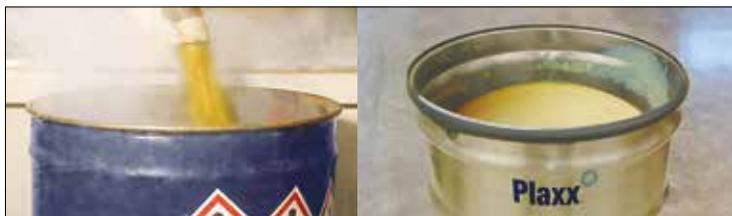
The chemically recycled plastic is broken down into oil and wax fractions. The company has forward sold all the oil and wax product from its first 12 machines to customers in polymer and wax manufacturing for further refinement
