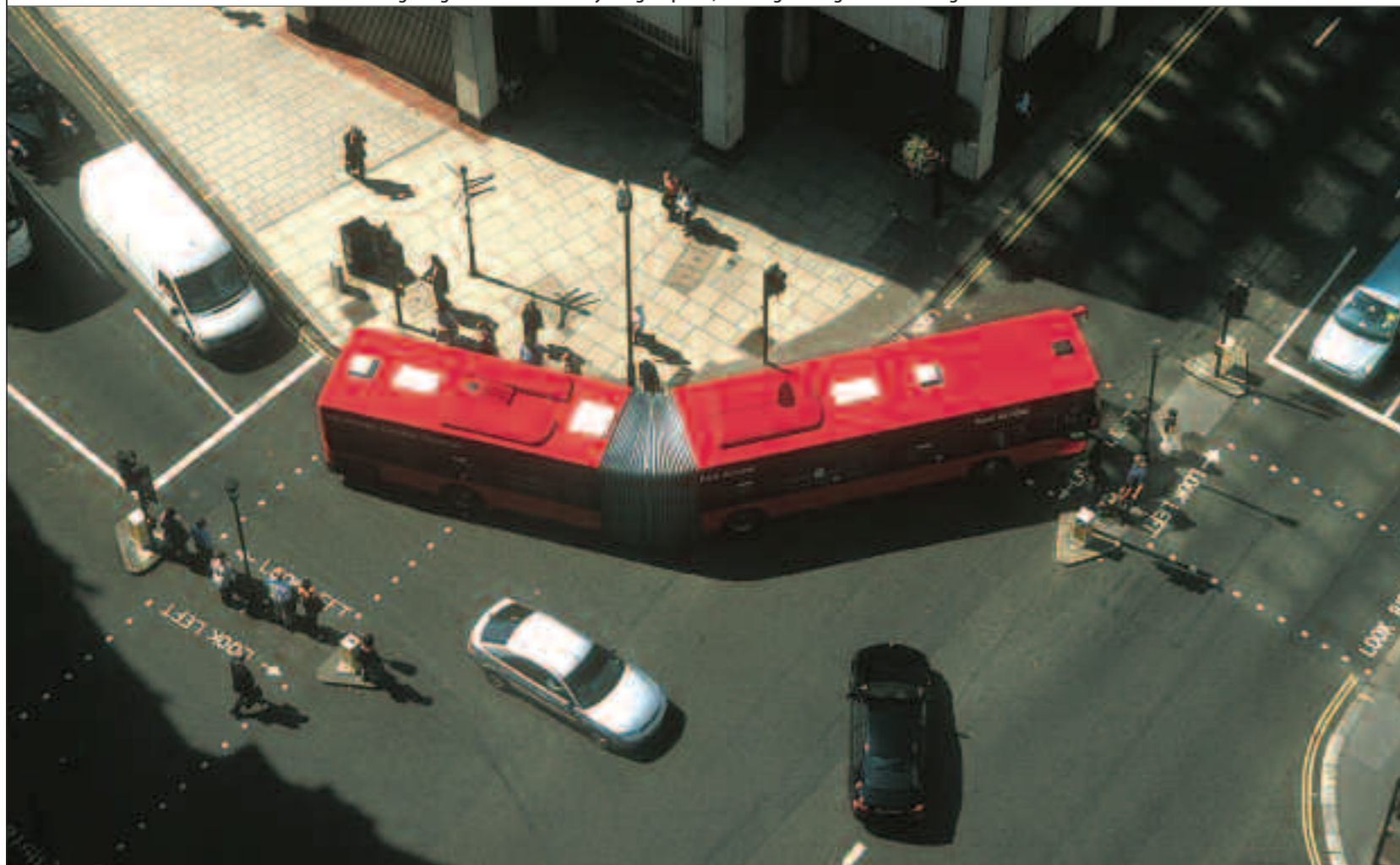
The short wheelbase of the front half of the vehicle gives good manoeuvrability in tight spaces, allowing the large vehicle to negotiate narrow roads © TfL
