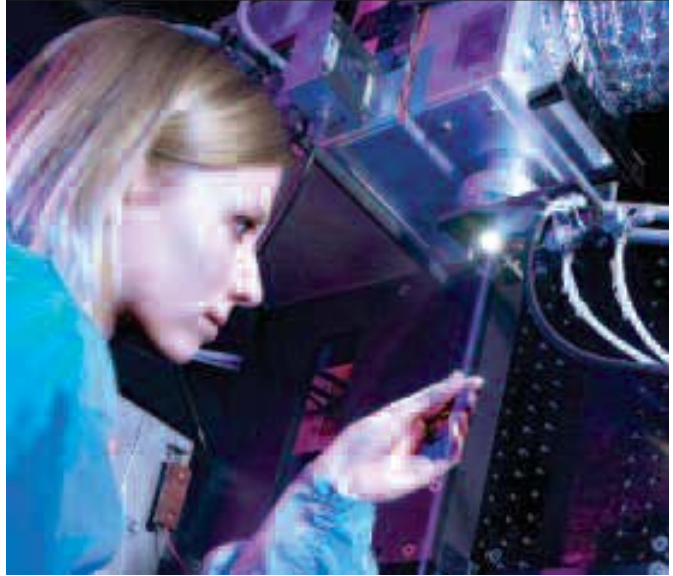
GTWave® fibre being inspected at the bottom of the fibre drawing tower © SPI
