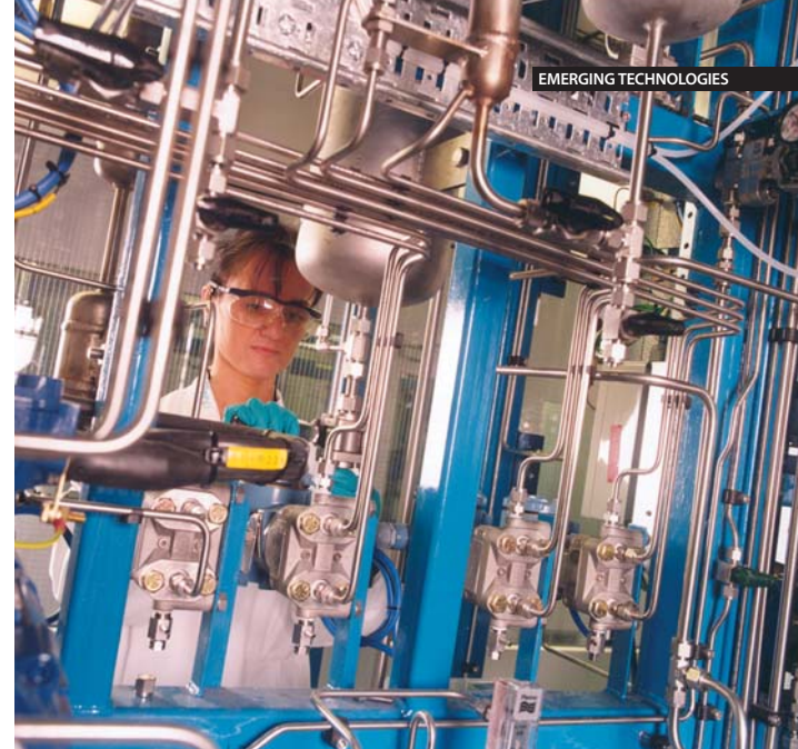
In the Davy Technology Centre, showing a section of the Mini-Plant which is used to process development and validation
