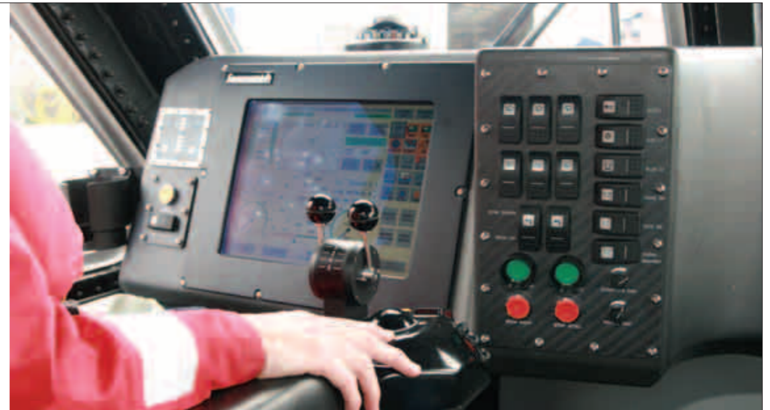
Seat-mounted controls and a flat screen enhance the ergonomics of the crew-members' position onboard © RNLI
