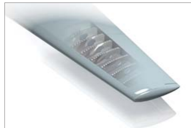
Schematic showing the ribs within a wing
