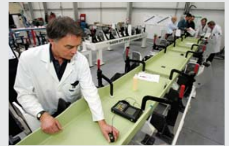
An engineer inspects the spar for de-laminations using an ultra-sonic probe © GKN Aerospace
