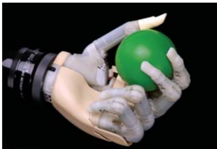
The i-LIMB Hand offers a range of different grip patterns for unparalleled dexterity
