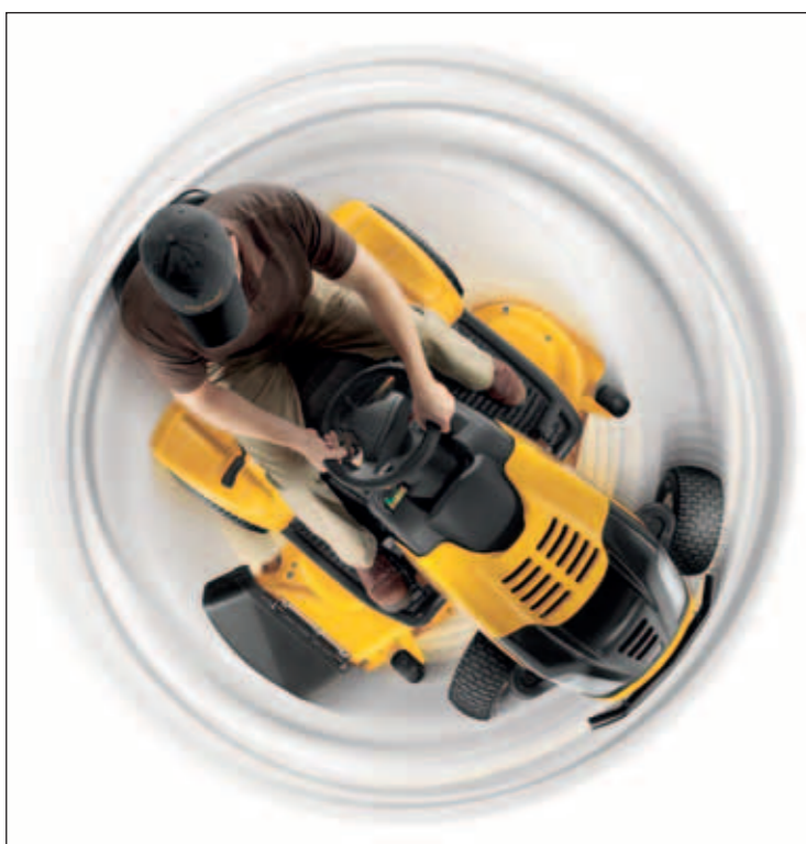
Figure 2a: Torotrak's zero-turn ride-on lawn mower transmission is already in production in the US
