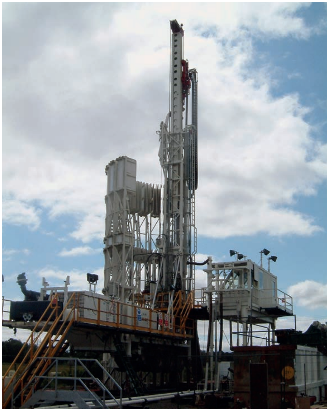
A modern drilling rig equipped for long-reach directional drilling in deep coal seams. The semi-circular rack behind the rig mast is an automated drill-pipe carousel © Paul Younger
