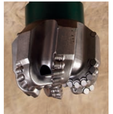
A polycrystalline diamond compact drilling bit used in directional drilling to cut rock. A high fluid flow rate through the bit and diamond tipped cutters ensure high rates of penetration can be achieved with efficient cuttings removal and stable directional performance to drill the well. Photo by www.jmdomke.com
