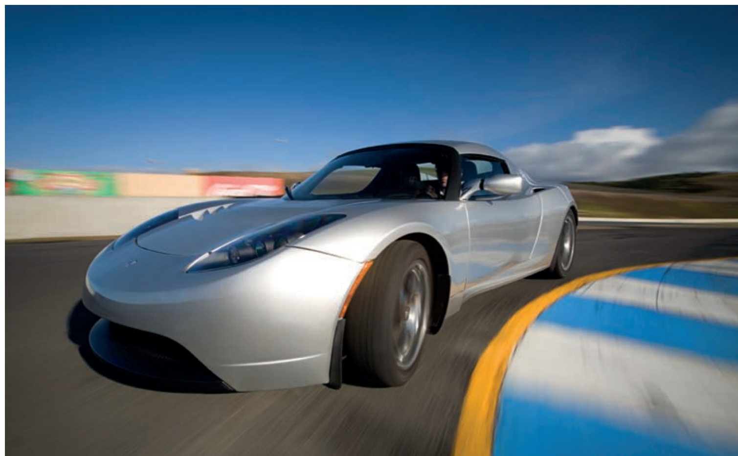
The Tesla Roadster, a sports car designed by Lotus Engineering and manufactured by Tesla Motors, uses a 375V, 53 kWh battery pack of lithium ion cells with lithium cobalt oxide chemistry providing a massive energy density of 120 kWh/tonne. Its battery can be recharged in 3½ hours, has a range of 236 miles and an expected lifetime of 100,000 miles or five years © Tesla
