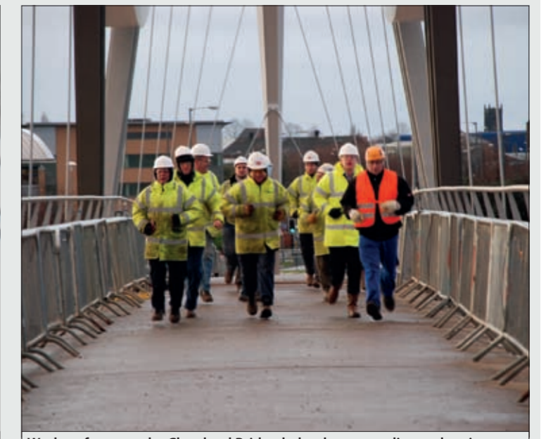
Workers from nearby Cleveland Bridge helped carry out live pedestrian testing of the bridge © Tim Harris, Expedition
