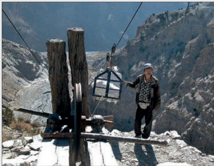
An upper station of a gravity ropeway installed in Janagaon, Nepal. Janagaon is one of six communities which have benefitted from this goods-transportation ropeway. The proven technique can now be copied elsewhere from a free technical brief available online.
