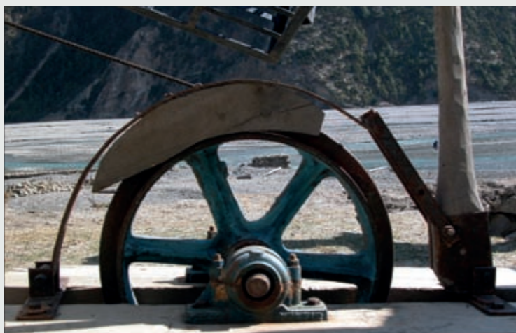
The braking system reflects the diagram in figure 3. When the lever on the right is pulled back it will pivot on the 6" bolt and cause the wooden block above the wheel to drop down, thus applying pressure and slowing the wheel speed.
