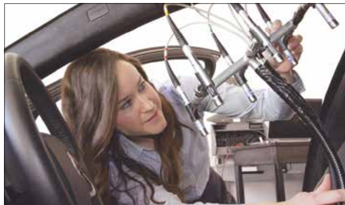
Orla setting up microphones that demonstrate the acoustic frequency response for typical listeners of different heights. Each pair of microphones represents a pair of ears
