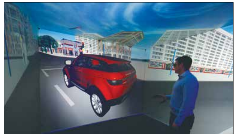
A 3D model of a Range Rover Evoque in Jaguar Land Rover's CAVE-like display. The computer simulations allow engineers to visualise full-size 3D models of components and the vehicle before physical parts are available © Jaguar Land Rover
