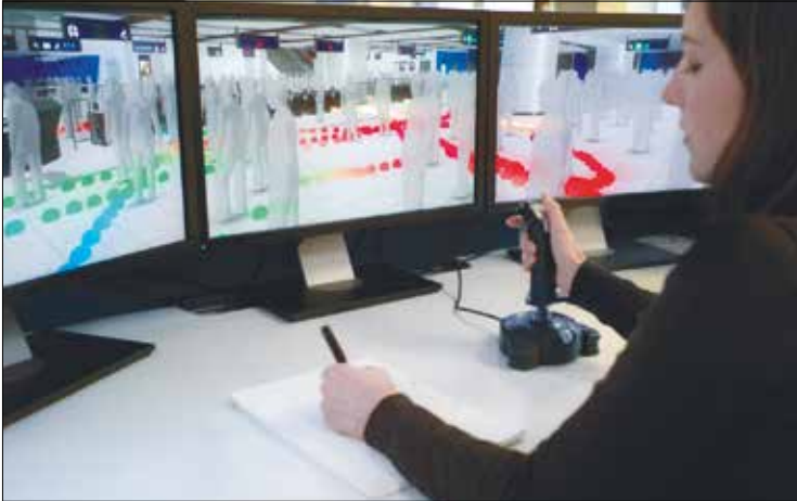
A prototype tool from Arup being used with a joystick interface to test the proposed signage at a large new underground rail station. The screens offer an accurate and realistic representation of the architecture and of a passenger's field of vision as the user walks through the virtual station. The lines of coloured spheres are traces of other virtual users, with colouring of the spheres indicating walking speed © Alvis Simondetti, Arup
