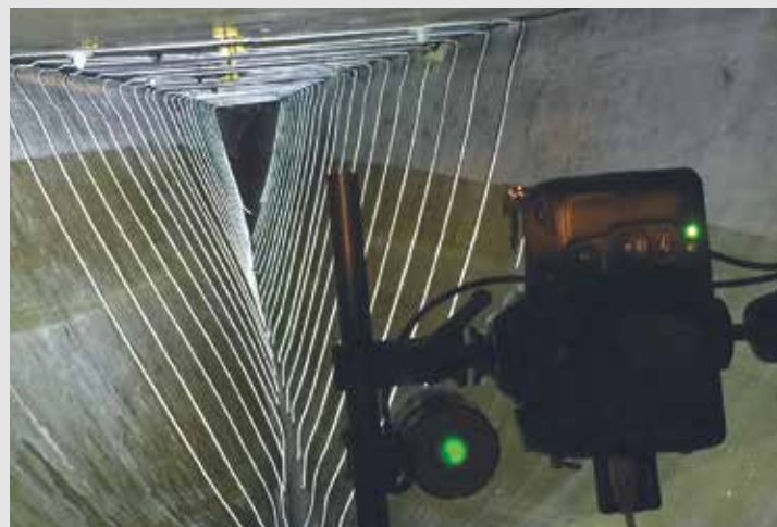
Optical condition monitoring takes place inside a wind turbine blade, using the digital image correlation system developed by ORE Catapult and Wideblue
