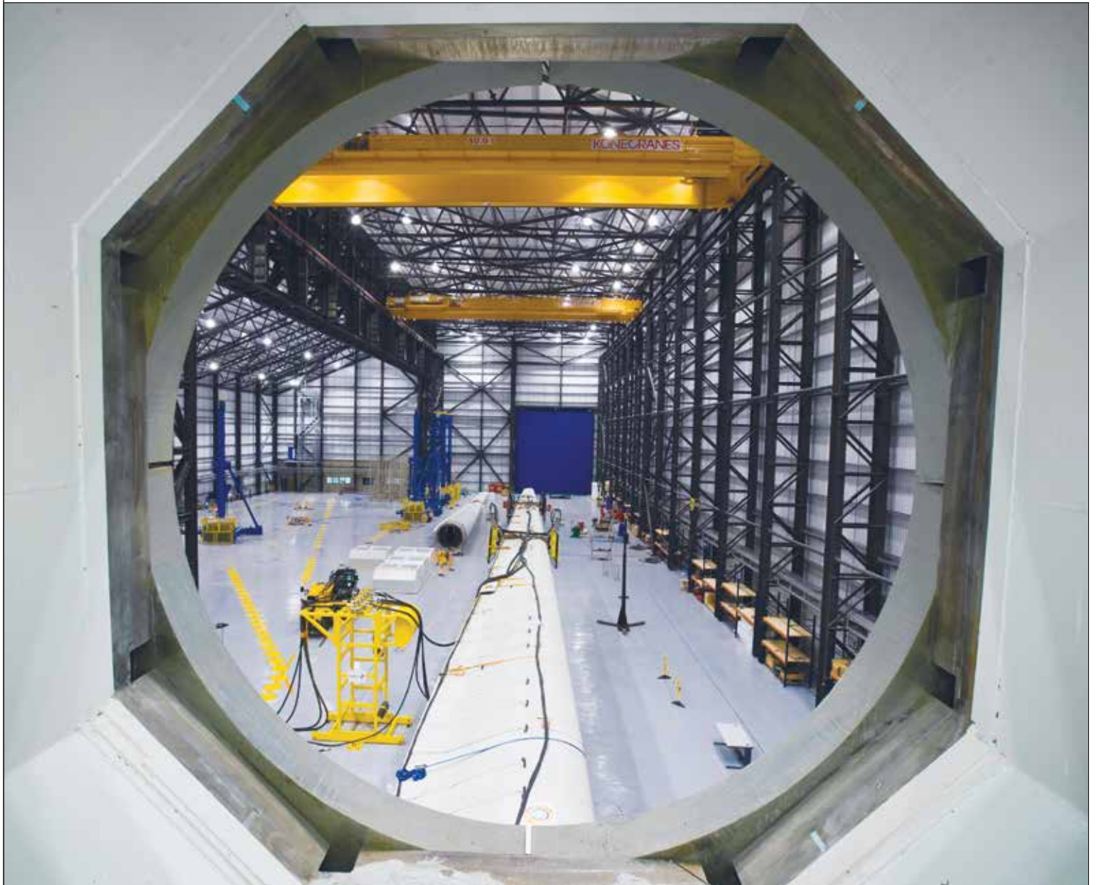
The facilities at the Offshore Renewable Energy Catapult are used to carry out tests on wind turbine blades up to 50 and 100 metres © HR ORE Catapult
