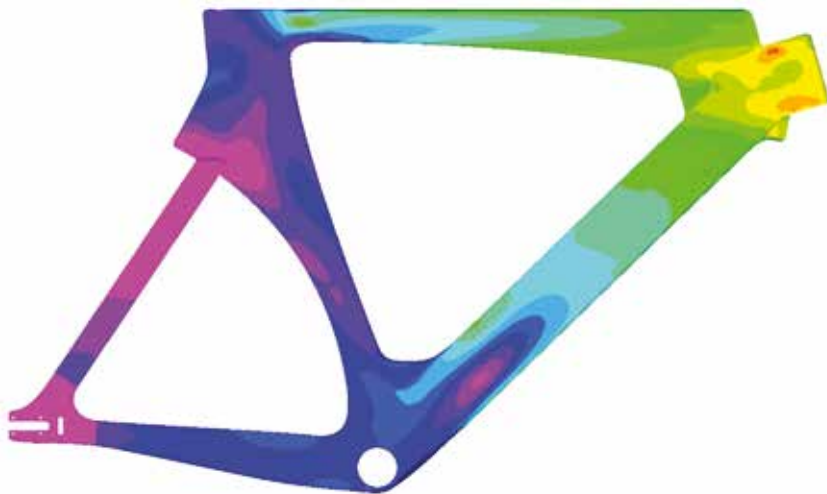
A finite element analysis (FEA) process was used to aid development of the T5GB frame. The T5GB achieves part of its performance benefit by having a shape that reduces aerodynamic drag. However, this reduction runs counter to the need to have frames that are structurally optimised for high stiffness and low weight. One of the advantages of the T5GB is that it incorporates those two contradicting requirements. This balance was achieved by using technical expertise and experience from motorsport and similar high-tech/fast-paced industries to engineer the optimal frame in a rapid timescale © Lentus Composites and Cervélo
