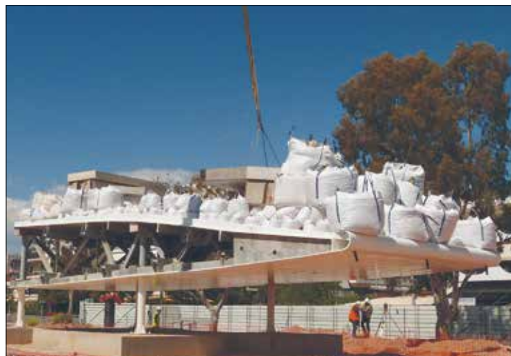
The prototype section of the canopy with its twin ferrocement shells and steel bracing being load tested in Athens. When the structure safely survived its anticipated failure loading, the team added concrete blocks to see when and how it would collapse, but they did not induce failure © Expedition Engineering
