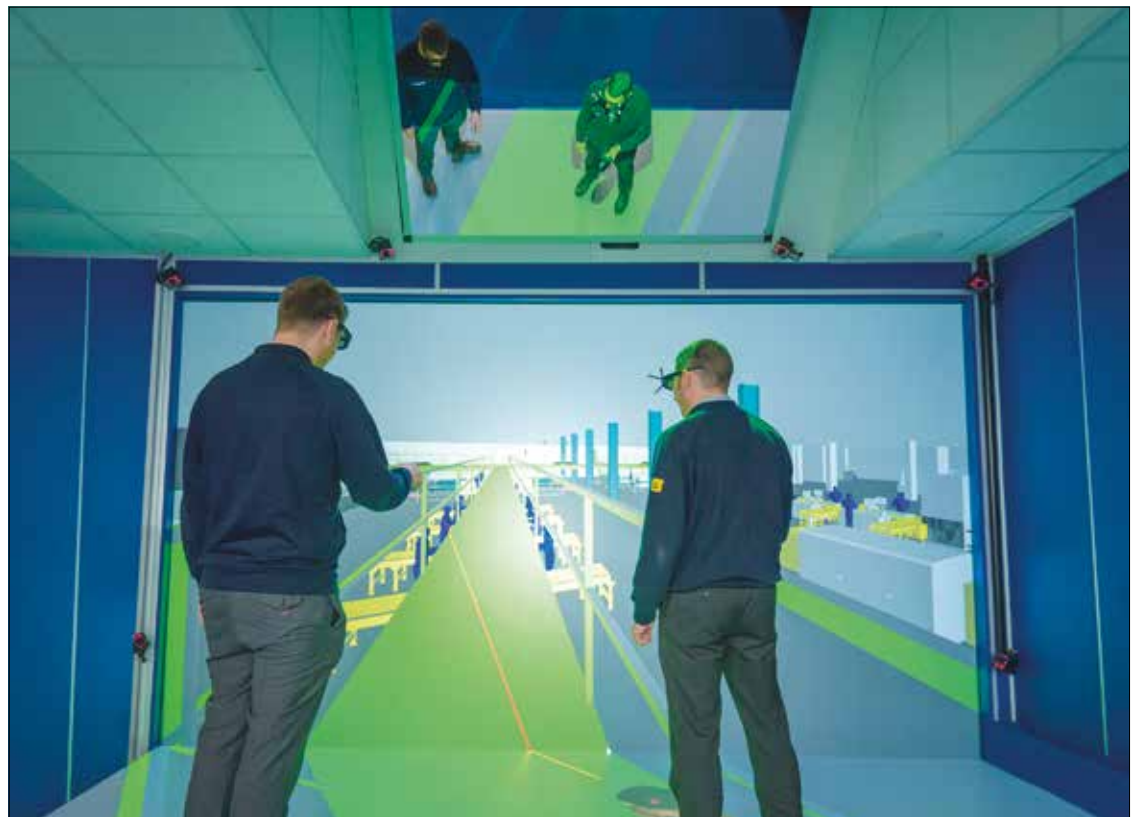
The Virtualis ActiveWall at Siemens' Congleton factory allows a group of operators, designers and engineers to work together when developing workcells for the assembly line © Virtualis
