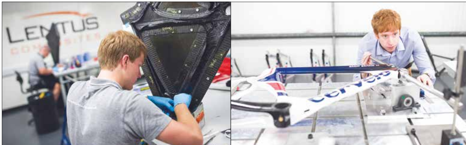
Left: Engineers place computer-cut plies into the mould tooling, based on the design that was developed through the FEA process. The placement of these plies is critical to achieving the desired frame stiffness and strength, so they have detailed instructions and diagrams to help. Right: An engineer tests the finished frame for stiffness at Lentus Composites. Multiple stiffness tests were carried out using methods that were developed by Cervélo, based on its knowledge of how frame stiffness relates to bike performance and rider feel. The test demonstrates that the T5GB will behave and handle in the way Cervélo intended
