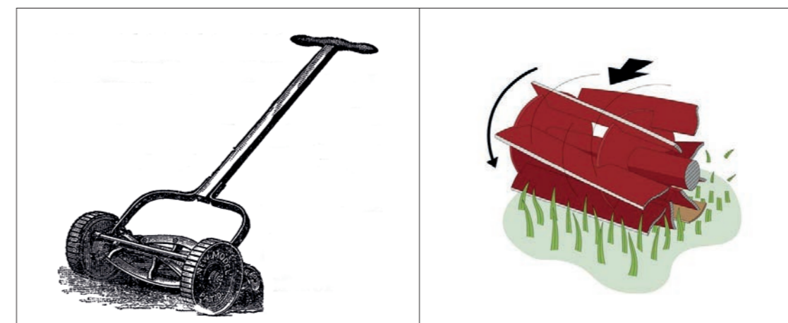
Left: Edwin Budding patented the cylinder lawnmower of 1830. This model is from 1888 © Wikipedia. Right: A cylinder mower's sharpened blade cuts across a fixed blade like scissors through paper © Allett Mowers
