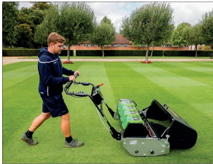
The Allett C34 Evolution weighs 160 kg with cartridge loaded and is balanced so that only 12 kg of downward pressure on the wide handle bar is needed to pull up the front end © Laura Malkin, Allett Mowers
