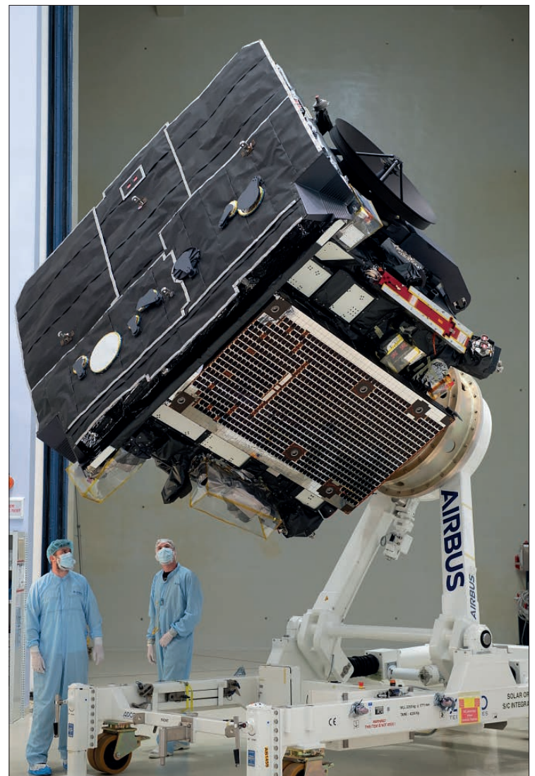
In October 2019, the Solar Orbiter had undergone a year's worth of tests near Munich. It is seen here being packaged up to be flown to NASA in Florida. The heat shield is shown on the left of the probe pointing upwards
