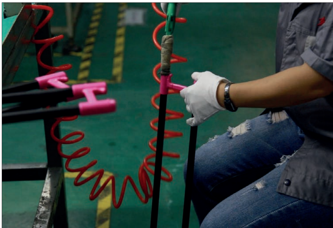
After a trombone slide has had the interior tube smoothed out by a solvent-based solution it is given a blast of compressed air to check that it is airtight © Warwick Music Group
