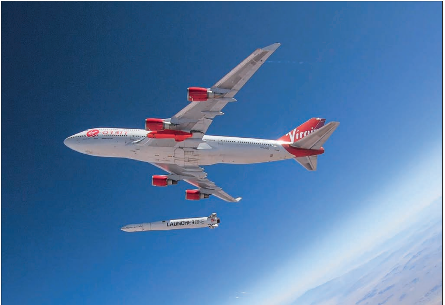
Virgin Orbit uses a modified aircraft to launch satellites into low Earth orbit © Virgin Orbit
