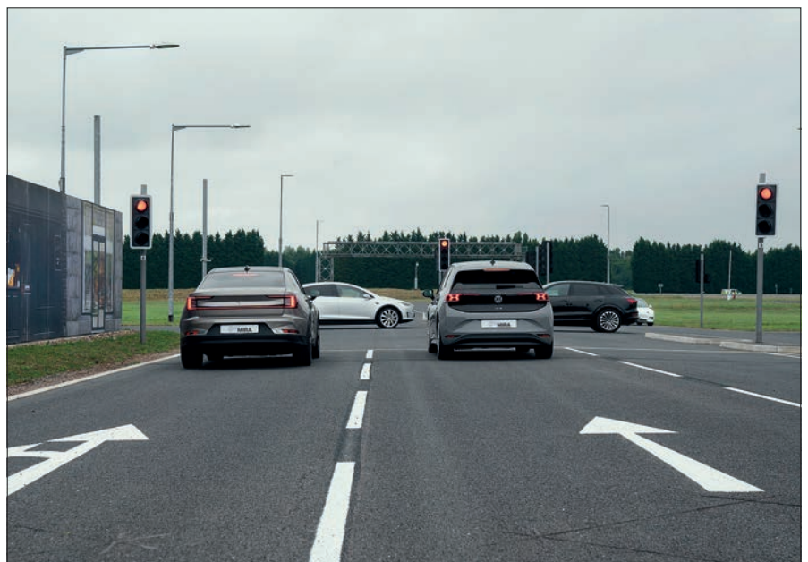
Urban and suburban driving environments can be recreated to validate complex automated driving systems under safe and repeatable test conditions © HORIBA MIRA
