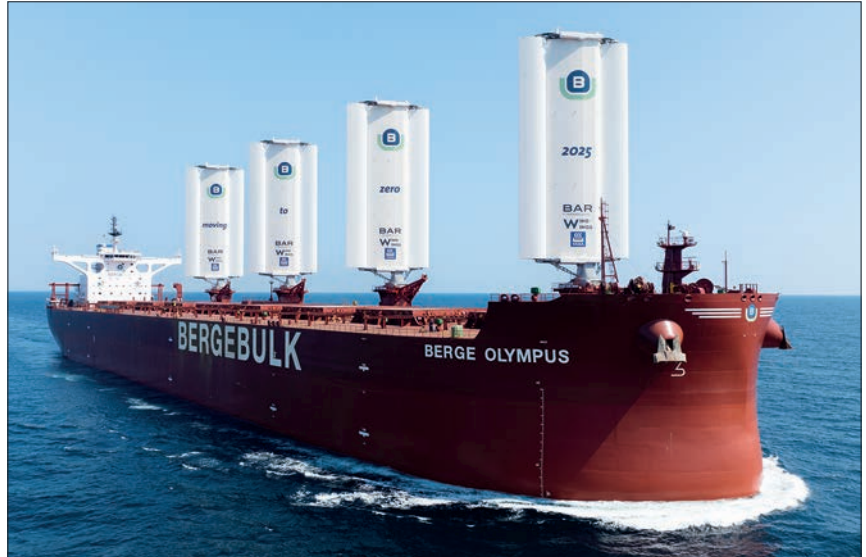
The Berge Olympus has four WindWings, saving 6 tonnes of fuel per day © BAR Technologies
