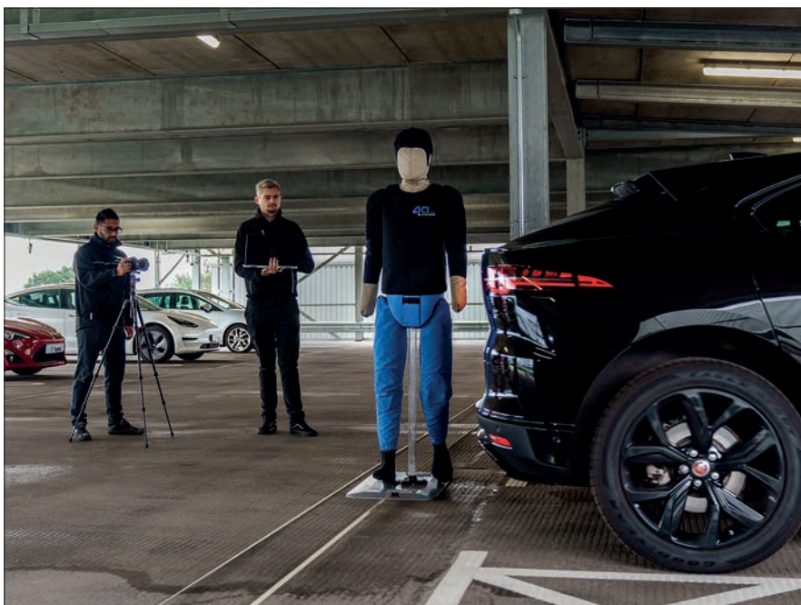
ASSURED CAV parking replicates the challenges of real-world situations to help develop self-parking solutions, allowing representations of vulnerable road users to be incorporated into test scenarios © HORIBA MIRA
