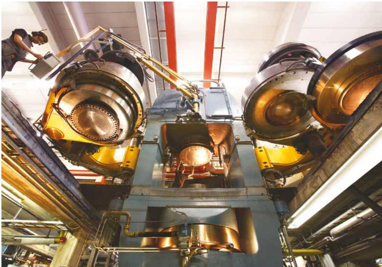
A large high-pressure high-temperature diamond press. Inside the module being lifted into the press (left, adjacent to operator) sufficiently high pressures and temperatures are generated to convert graphite into industrial diamond © Element Six
