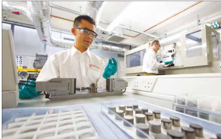
**Synthetic diamond oil and gas cutters under analysis at Element Six's Global Innovation Centre. The engineer is holding a cylinder manufactured by sintering diamond powder (at high temperature and pressure) on a tungsten carbide substrate. Many such disks are mounted in a drill bit (the teeth) for drilling through rock © Element Six**
