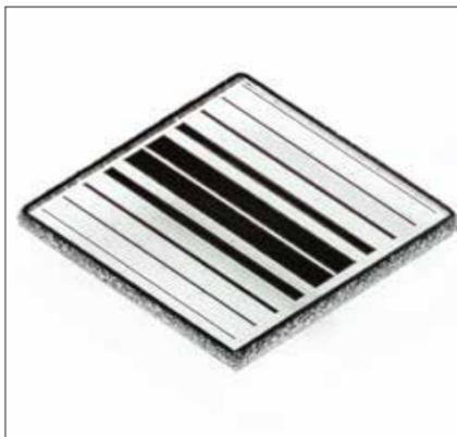
**An intrinsic piece of polycrystalline CVD diamond (colourless) into which has been grown boron-doped electrically conducting diamond bands of different widths. The chemical resistance of the all-diamond device means that the conducting diamond band electrodes can be used as sensors, even in highly corrosive environments** Picture taken by Dr Jon Newland; device fabricated by Element Six Ltd and the University of Warwick
