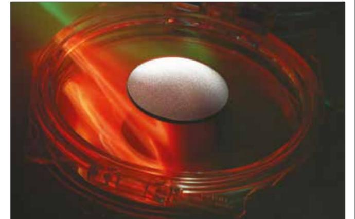
**An unmounted synthetic diamond tweeter dome approximately 25 mm across (manufactured by Element Six) sitting in a membrane box and used in Bowers & Wilkins speakers © Element Six**
