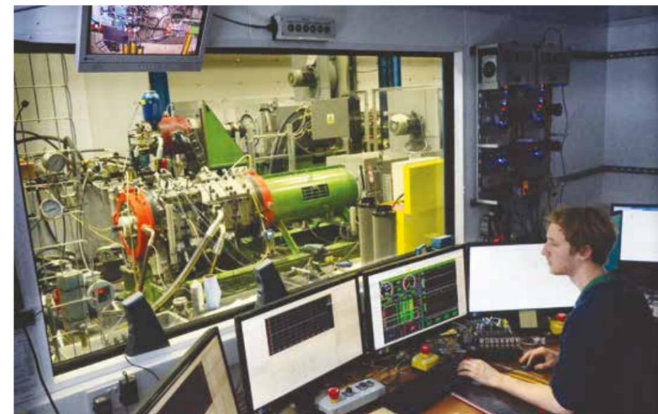
Testing the performance of a 1.5 MW Digital Displacement® motor
