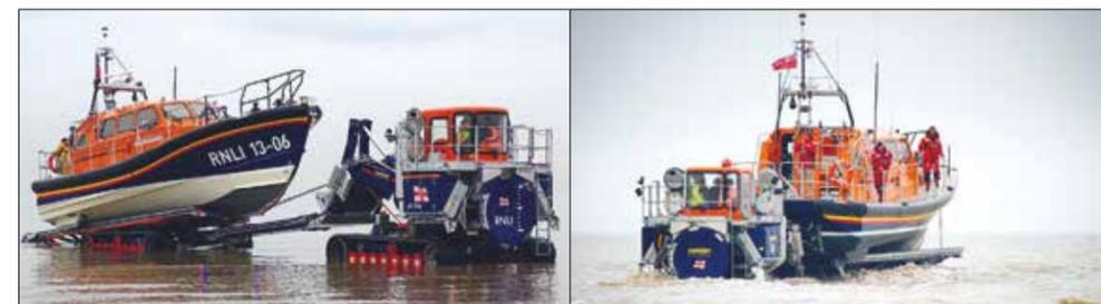
The Shannon can be recovered from the sea by the launch and recovery tractor. The boat sits on a 'slewing ring' that can be turned 180 degrees to relaunch the boat almost immediately © RNLI
