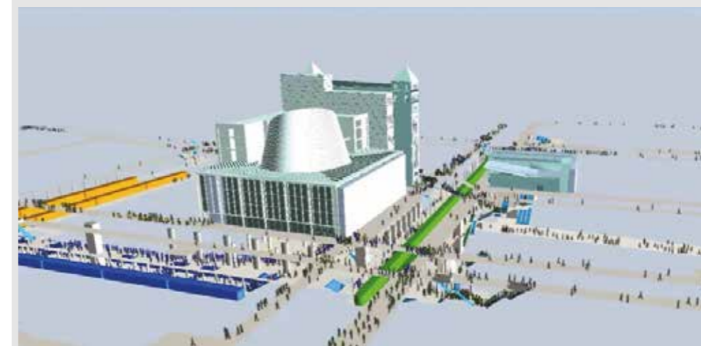
Fulton Center – looking south. Analysing pedestrian movement in Lower Manhattan. The Center is seen in pale green-blue with the World Trade Center site to the right of the image. The green, blue and yellow blocks represent subway trains stopped at the station © Arup
