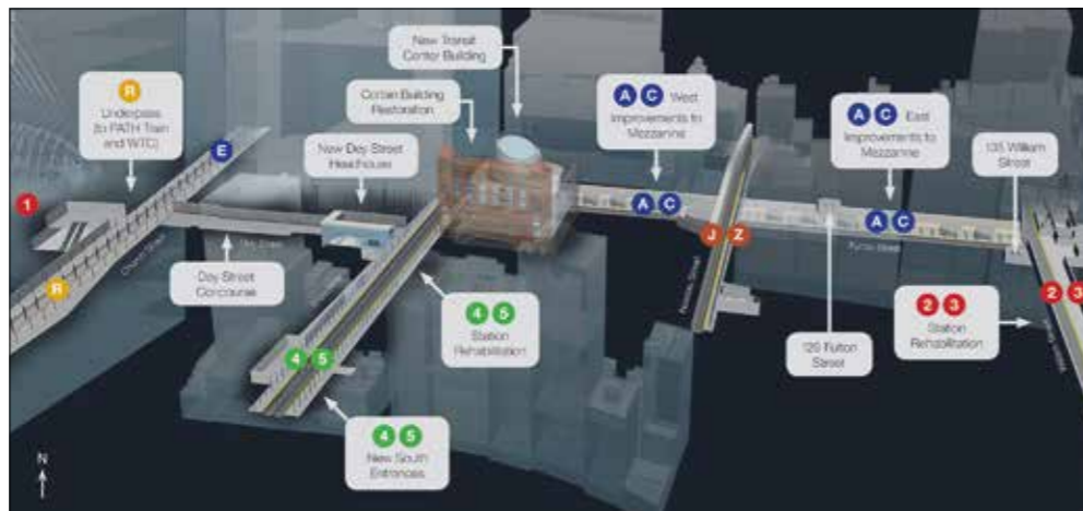
How the new Fulton Center interconnects six subway stations on 11 lines. Running north-south is the oldest and busiest route, the 4 and 5 Lines, built in 1902, which separates the new Day Street concourse from the new Transit Center building with the Corbin Building in front. Running east-west is the newest and deepest, the A and C Lines constructed as cast iron tubes in 1933, with a large cut-and-cover mezzanine above © Arup
