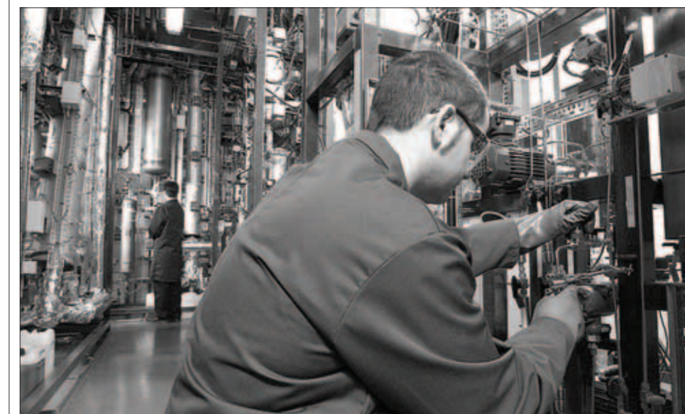
Lucite International's Alpha pilot plant is located at Wilton, UK. It fully reproduces the plant that was commercialised in Singapore in 2008 but at 1/25,000th of that scale. It is manned by two operators and one analyst 24 hours a day, 330 days a year. Lucite continue to run the pilot plant to test improved catalysts and process enhancements and to develop the next generation of MMA technology based on the Alpha chemistry © Lucite International
