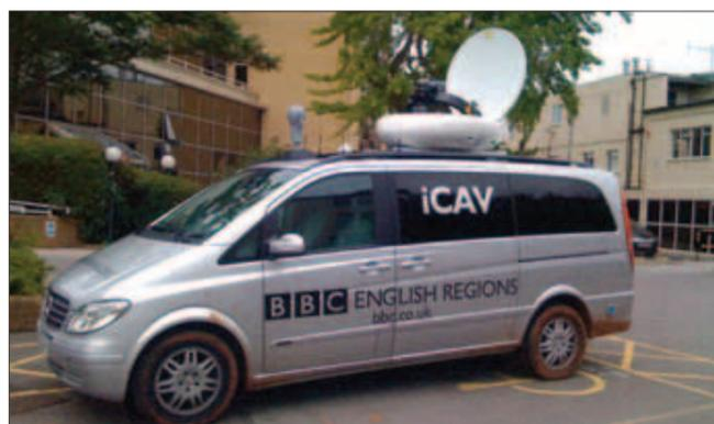
The iCAV is the first BBC vehicle capable of delivering direct, live video streams for the web. Built into a standard people carrier, it has DC powered internal batteries that means it can run for six hours without need of a generator © Matthew Sylvester
