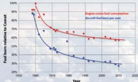
Figure 1. Aircraft fuel efficiency – past and predicted. Rolls-Royce schematic drawn by Simon Routstone
