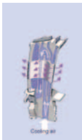
Figure 5: Cutaway of an HPT blade.
