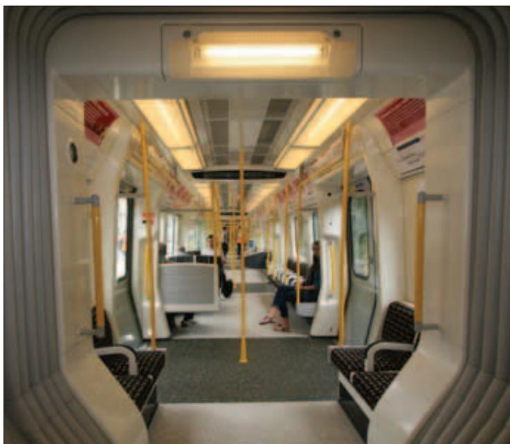
London Underground is introducing air-conditioned trains on the shallower sub-surface lines. By 2016, 40% of the Tube network will use the S-Stock Tube trains, which have saloon air conditioning. These trains have the first walk-through gangway carriages on the Underground. The inside of the train is one continuous length, providing improved capacity, security and passenger flow
