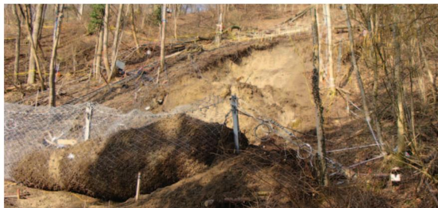
At the Rüdlingen monitoring site in the Zurich Canton an instrumented test field has been established to create and measure landslides. In this picture a Geobrug net has caught an induced landslide
