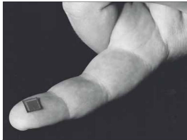
CMOS sensors paved the way for smaller cameras and the development of the 'camera on a chip'. Although not as high quality as CCD sensors, they use less power and are cheaper to produce. They are also integrated into fingerprint recognition on smartphones and are used for identification in biometric passport booths for border control
