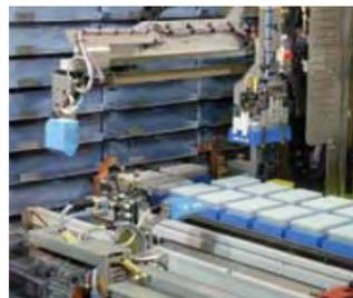
Racks of samples are stored on shallow insulated drawers. Drawers are accessed and racks are picked and placed robotically © The Automation Partnership
