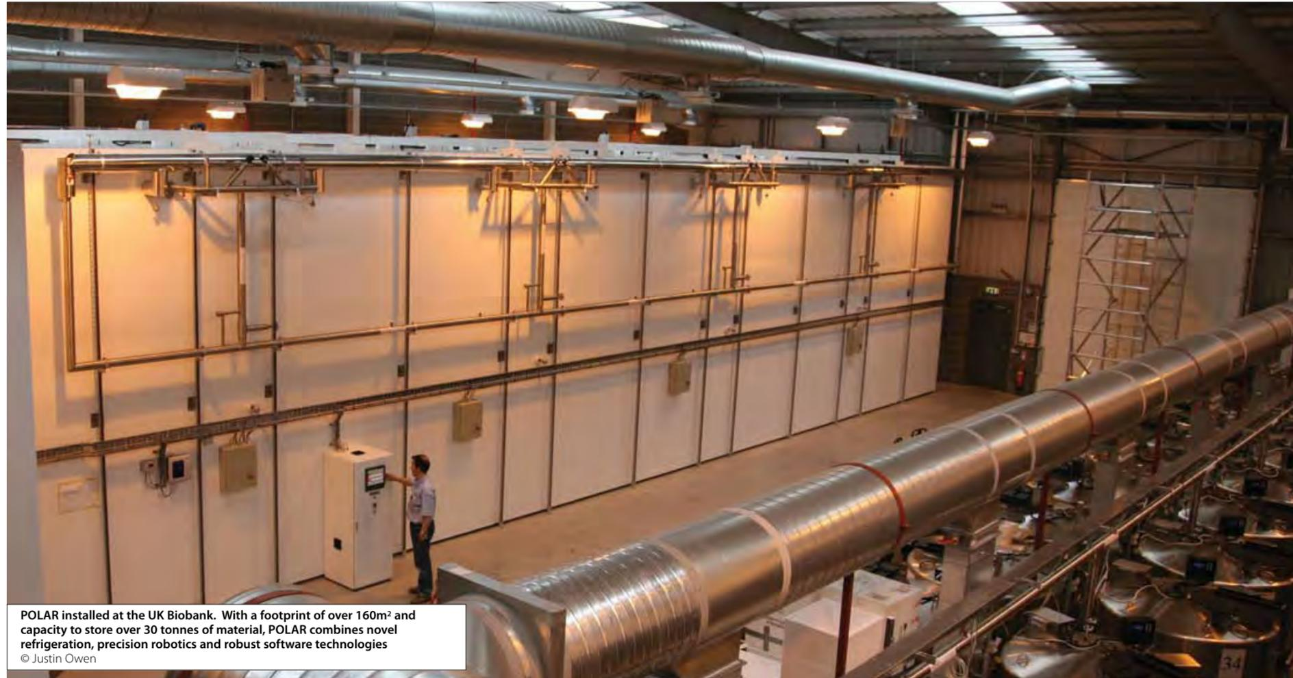
POLAR installed at the UK Biobank. With a footprint of over 160m<sup>2</sup> and capacity to store over 30 tonnes of material, POLAR combines novel refrigeration, precision robotics and robust software technologies
