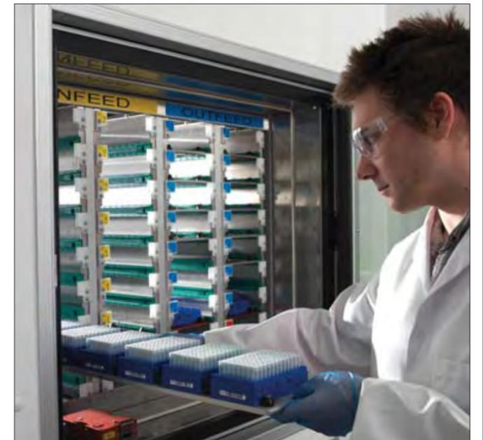
Biobank samples are physically protected and can only be sourced by an authorised user. Operators are not exposed to ultra-low temperatures and work in a conditioned antechamber. The loading and unloading is safe and ergonomic and incoming samples are held at -20°C while awaiting transfer to storage © The Automation Partnership
