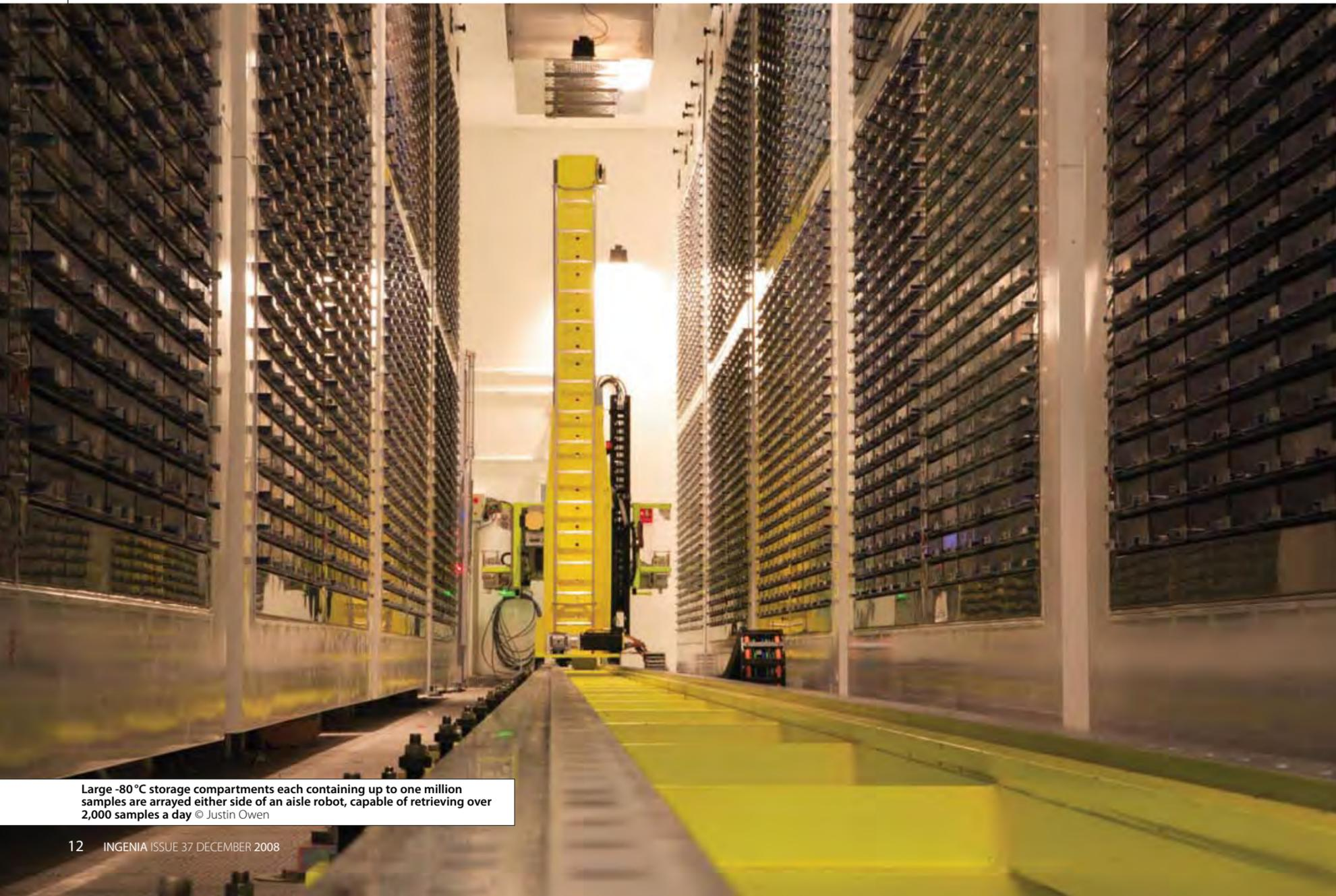
Large -80°C storage compartments each containing up to one million samples are arrayed either side of an aisle robot, capable of retrieving over 2,000 samples a day © Justin Owen
