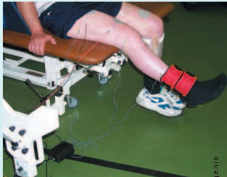
**Figure 3: Experiment illustrating closed-loop control of knee-joint angle via FES**
