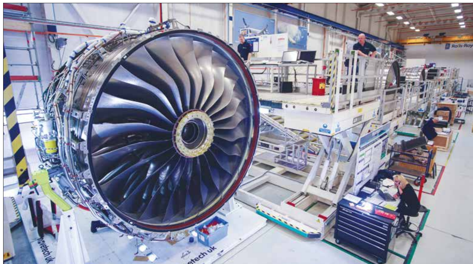
University of Oxford research on computational fluid dynamics (CFD) helped Rolls-Royce design its Trent 1000 and newer Trent XWB engines (pictured here). Researchers from the Numerical Analysis Group initially developed the HYDRA CFD package, which allowed Rolls-Royce to use CFD codes to simulate the flow of fluids in and around all products, including the flow of air through all components of diesel or gas turbine engines and their installations. Since 2009, HYDRA has become the standard aerodynamic design tool used across Rolls-Royce © Rolls-Royce
