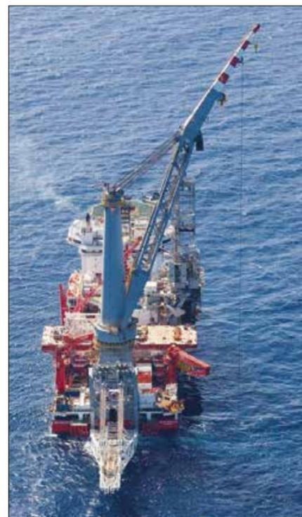
Stern view of a new breed of heavy construction vessel that can house a crew of 400. This ship, shown undergoing sea trials, is equipped with a large crane for lowering a 1,000 tonne structure to the seabed up to 1,000m below sea level. It can also lay flowlines in ultra-deep water using both the S-lay and J-lay techniques. It is considered to be a \$0.5 billion multipurpose solution for the global deep water SURF market
