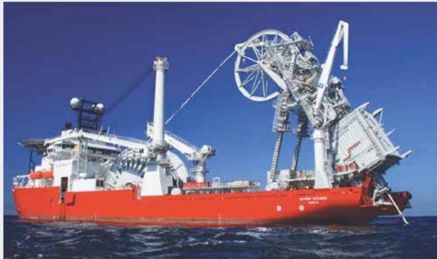
A reelship laying a flowline at sea. When loaded onshore, the flowline is plastically strained as it is spooled on the reel. When offshore, the process is reversed and the flowline passes through a three-point straightener before being laid via tensioners positioned on a variable-angle ramp. The technology is extremely efficient for the relatively short flowlines used in the hub-and-spoke architecture in the North Sea SURF market © Subsea 7
