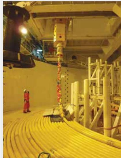
A subsea control umbilical being loaded into a large storage carousel located within the cargo hold of an offshore construction vessel. These specialist ships are able to automatically load umbilicals, many kilometres in length and several thousand tonnes in weight, at the quayside and accurately lay them on the seabed offshore. Remotely operated vehicles or divers then connect them to production hardware on the seabed
