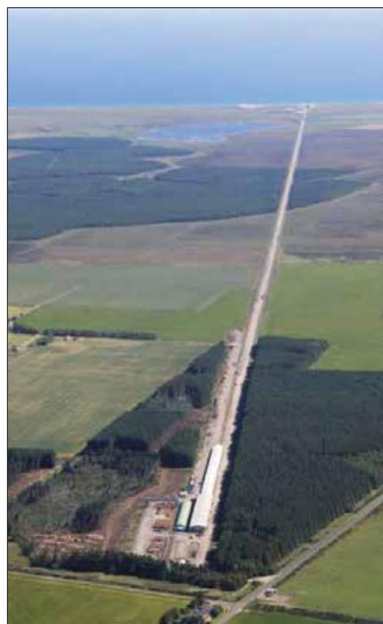
A Subsea 7 fabrication site at Wick produces several flowline bundles a year weighing thousands of tonnes, which are then towed out to their subsea destinations. Welding pipelines together onshore reduces the need for heavy construction vessels offshore. Large prefabricated subsea manifold/tow-head structures at each end of the bundle enable the testing and commissioning of the complete system onshore, thereby reducing the time for bringing the oilfield on-stream offshore
