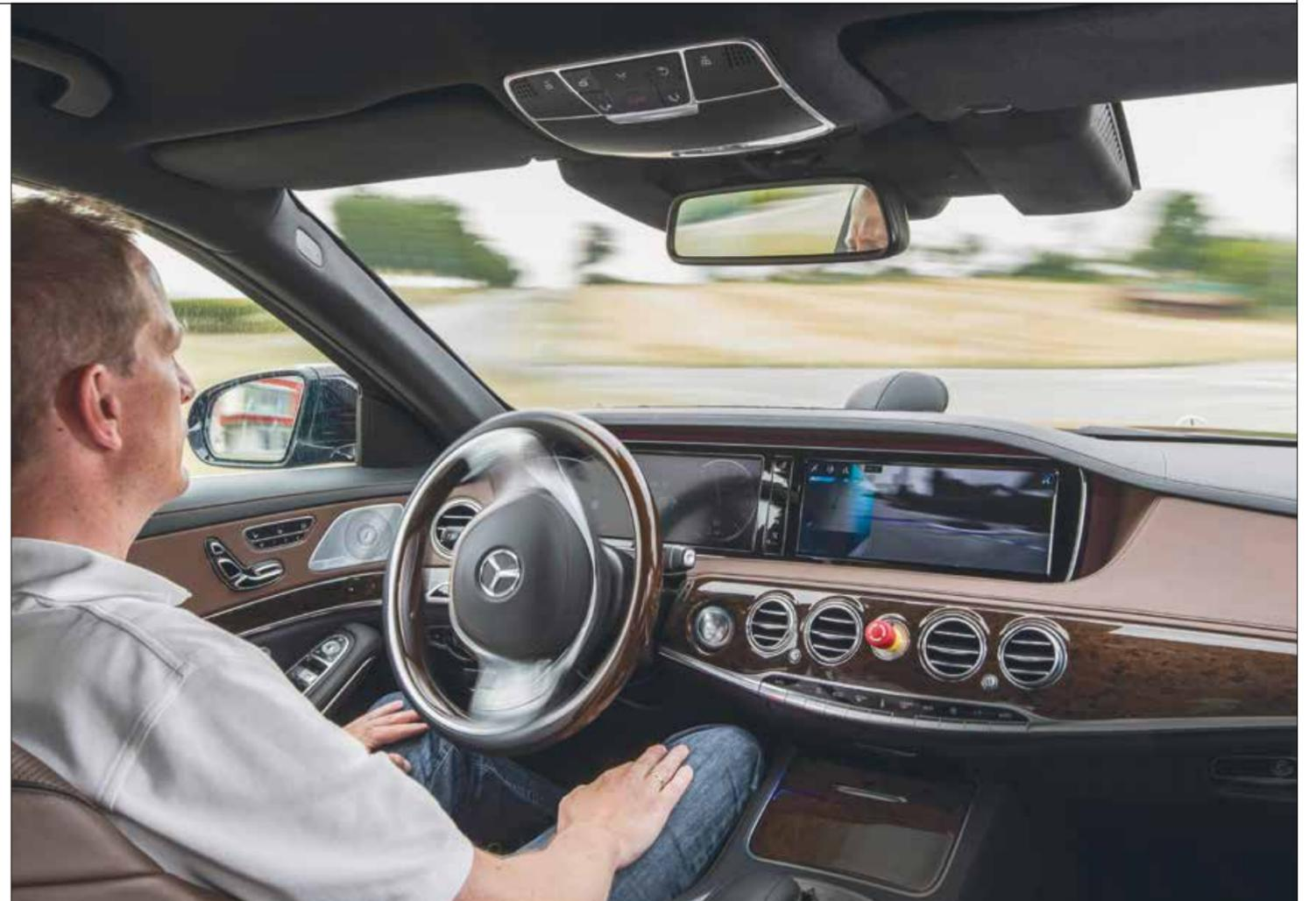
The new Mercedes S 500 autonomous car uses sensors already fitted on the production S-Class to 'see' obstacles and interpret roadside information and a sophisticated route pilot to navigate the way. In September 2013 the pilot car took on traffic lights, roundabouts, pedestrians, cyclists and trams, as it navigated its way from Mannheim to Pforzheim, in western Germany
