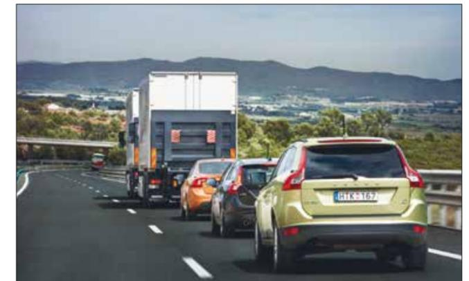
In May 2012, Europe's first ever autonomous vehicle road train took to the road outside Barcelona, Spain. The convoy of autonomously driven Volvo vehicles followed behind a lead vehicle driven by a professional driver. The five vehicles drove on a public motorway among other road users at 85 km/h, with a gap between each vehicle of 6m. During the three-year project the vehicles drove a total of 11,000km © Ricardo
