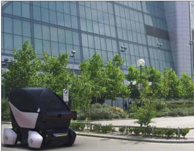
By mid-2017, it is planned that 100 fully autonomous cars will be operating in Milton Keynes, sharing pathways with pedestrians and equipped with sensors to avoid collisions. The LUTZ (Low-carbon Urban Transport Zone Pathfinder) driverless pods, which can carry two people each, will be able to travel at a maximum speed of 24km/h © Transport Systems Catapult
