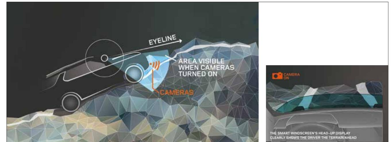
Transparent bonnet technology is one of the technologies being developed for the Land Rover Discovery
