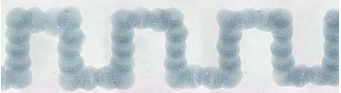
creating a package similar to a seal sticker. If the grid is printed on a brittle layer sandwiched between softer epoxy layers, any strong force applied to the chip will lead to the brittle layer cracking and breaking the protection grid, safeguarding the device. Further, if the criminal tries to pick off the resin coating around the chip, the grid that sits within the plastic is physically broken, rendering the device secure.
