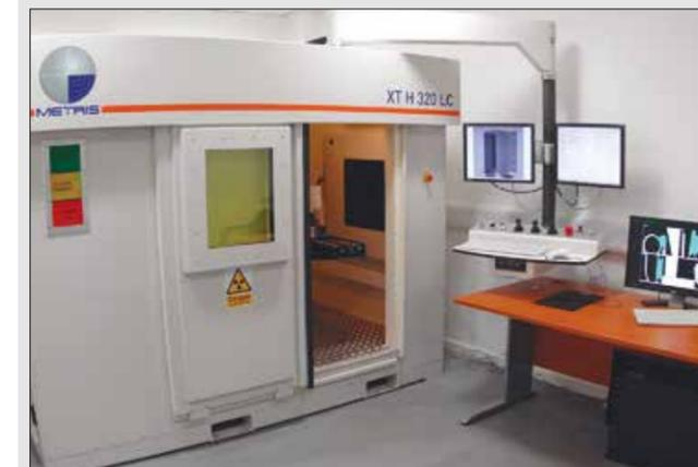
**WMG's micro-CT scanners enable cone beam X-ray sources ranging from 160 kV–320 kV, a voxel special resolution down to sub-micron levels (170 nm, 1 x 10–9 m), and a maximum sample size of 300 mm in diameter**
