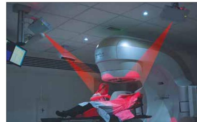
Ceiling-mounted AlignRT camera units map the surface of a patient's body to ensure that radiotherapy beams are correctly delivered and paused if the patient makes any slight movement © Vision RT
