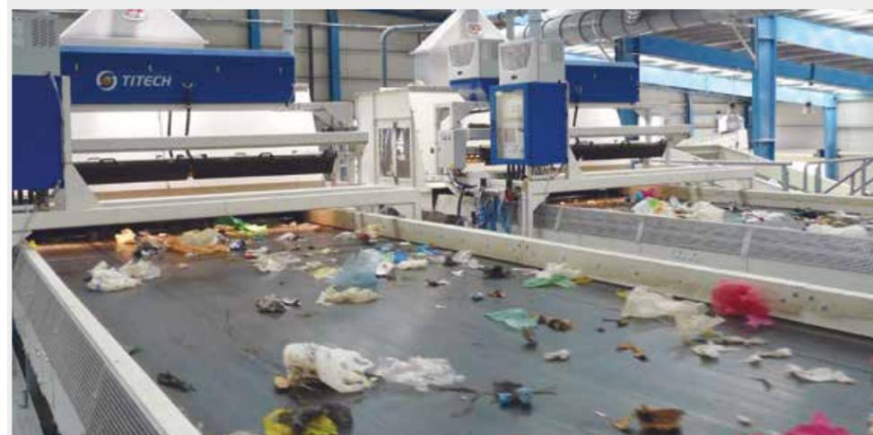
Infrared separators are the final mechanical stage of the materials refinement process, following stages such as prescreening by trommel, magnetic and air classification. In the photograph, waste is travelling on the conveyor from right to left where the sorting system is separating different types of plastic © Professor S R Smith
