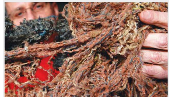
The company InterfaceFLOR plans to close the lifecycle loop with ReEntry 2.0, a process that recovers every component of carpet tiles, all of which can be made into new carpet tiles. This includes recycling nylon yarn, the most carbon-intensive part of the carpet © InterfaceFLOR
