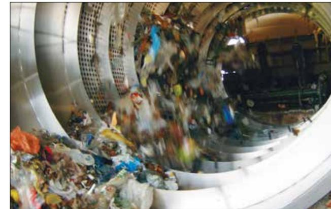
Trommels weighing around 20 tonnes filter materials into different size fractions at the beginning of the recycling process © Alex Marshall, Clarke Energy Ltd/Wikimedia Commons
