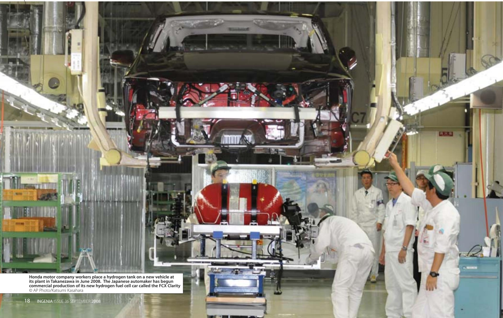
Honda motor company workers place a hydrogen tank on a new vehicle at its plant in Takanezawa in June 2008. The Japanese automaker has begun commercial production of its new hydrogen fuel cell car called the FCX Clarity © AP Photo/Katsumi Kasahara
