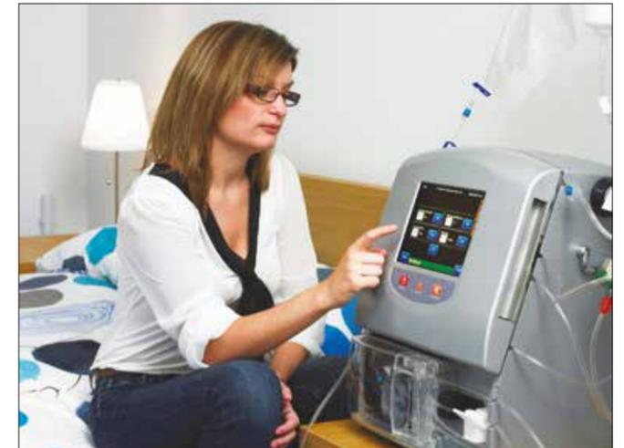
The Quanta SC+ is a portable single pass haemodialysis system that uses a disposable cartridge to generate the dialysate for every treatment. As the machine itself is never in contact with blood or the treatment fluids (the pre- or post- dialysis dialysate), it does not need disinfection or sterilization. © Quanta
