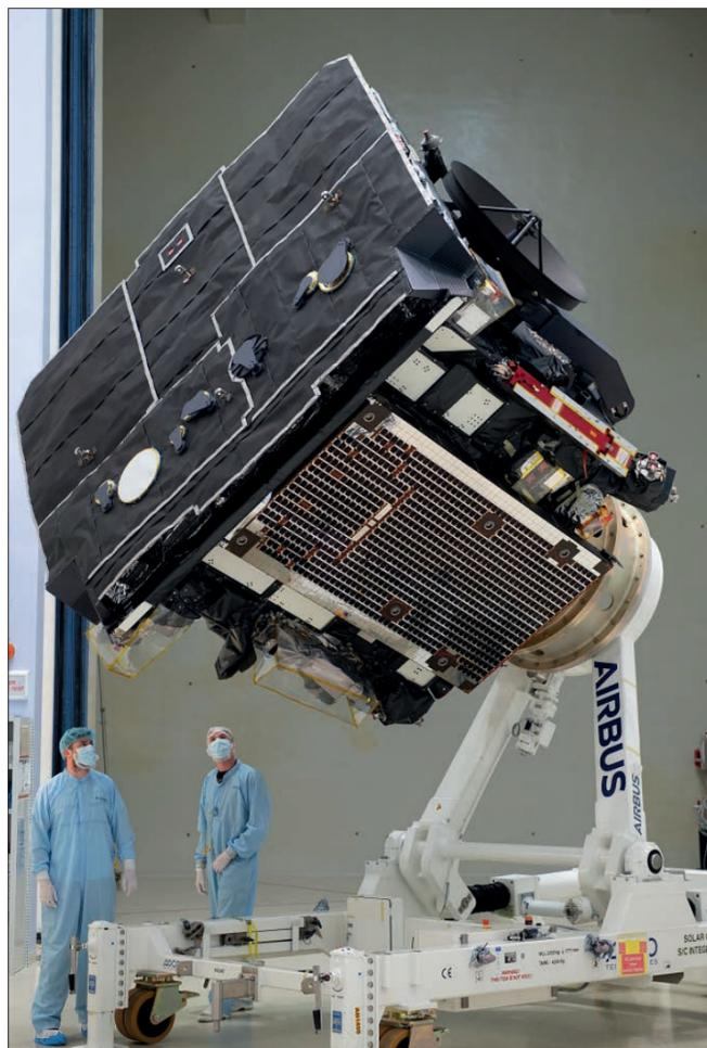
In October 2019, the Solar Orbiter had undergone a year’s worth of tests near Munich. It is seen here being packaged up to be flown to NASA in Florida. The heat shield is shown on the left of the probe pointing upwards © ESA – S Corvaja
