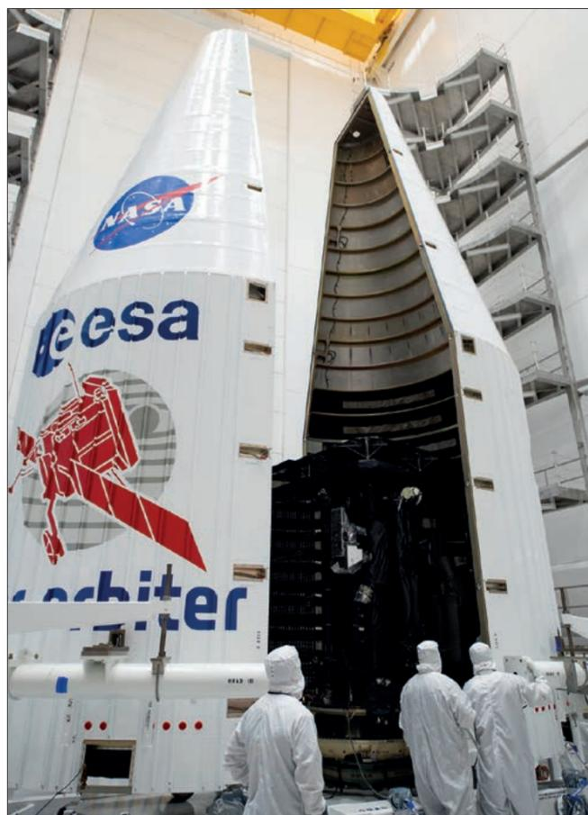
Solar Orbiter being encapsulated within the NASA rocket nose cone in February 2020 © ESA/ATG medialab
