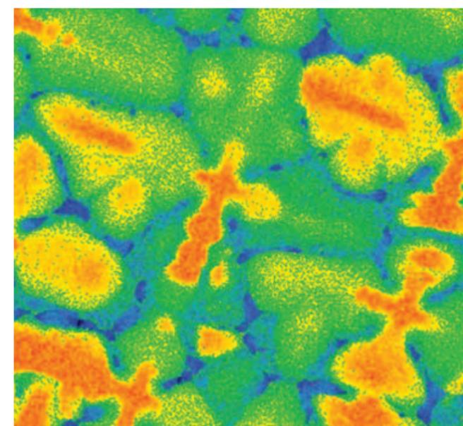
Maps of chemical elements in cast superalloys developed by the Cambridge UTC. Rhenium (top) and tantalum (bottom) are added to provide additional strength to the matrix and precipitates in these alloys respectively. When these alloys are cast, the rhenium partitions to the growing solid and tantalum partitions to the liquid, leaving the patterns shown above © University of Cambridge
