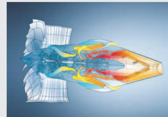
An intercooled/recuperative engine, one of four different core engine architectures that the NEWAC research programme looked at. This one uses heat exchanger modules in the main exhaust to extract thermal energy and transfer it back into the combustion chamber. NEWAC is aiming to reduce the fuel consumption of engines by 6% by improving core engine technologies and with it carbon dioxide emissions too © MTU Aero Engines
