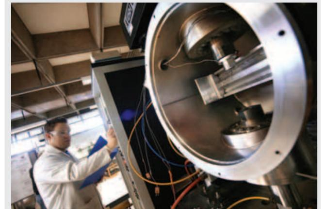
A test set up in the Metallurgy laboratory high temperature vacuum test chamber. It is used for the measurement of fatigue and crack growth data for high temperature (usually turbine) alloys © University of Birmingham
