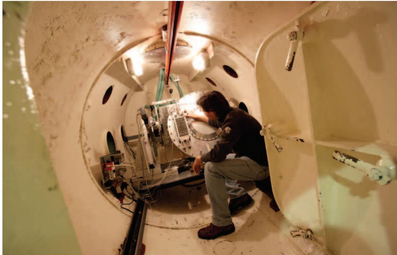
A senior researcher setting up a Low Pressure Turbine 'cascade' experiment in the Whittle lab – a high speed airflow facility that allows detailed testing of turbine aerofoil geometry to determine the aerodynamics of the blade sequence at engine representative conditions © University of Cambridge
