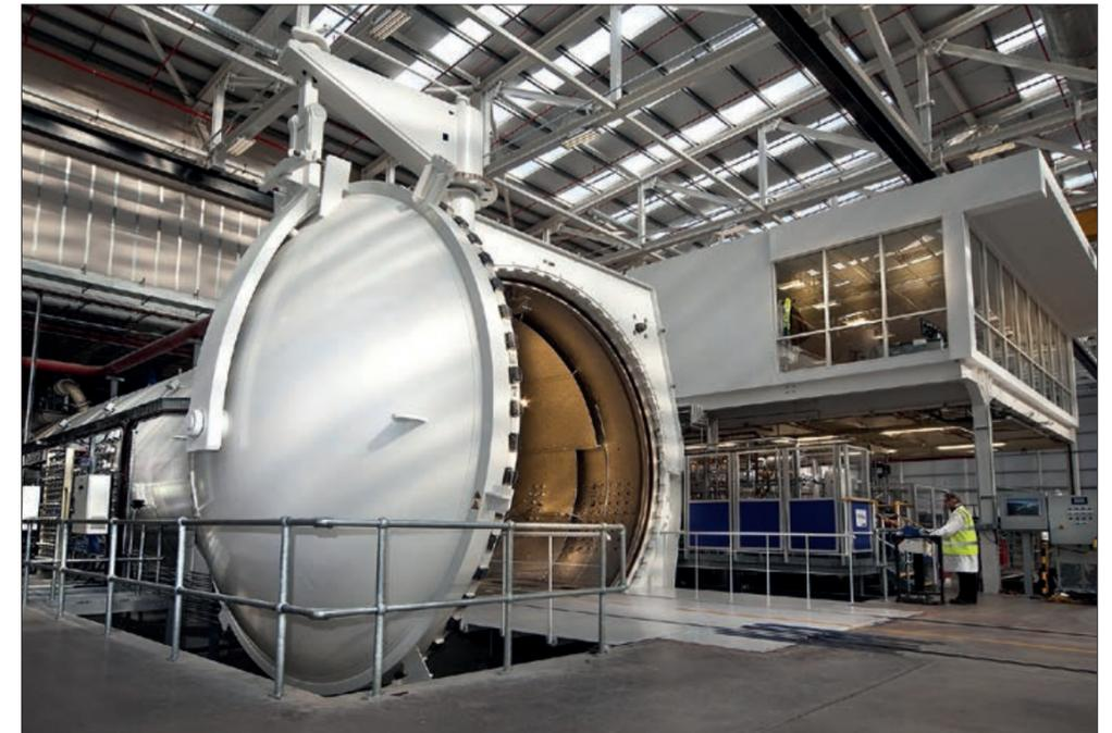
The autoclave area in the Wing Manufacturing and Assembly Facility at Bombardier Belfast where the wings are cured © Bombardier
