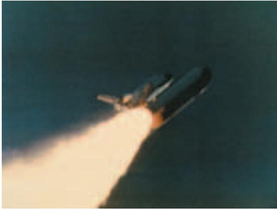
**The Challenger space shuttle in flight just before failure; a small flame can be seen at the site of the booster seal leak.**
