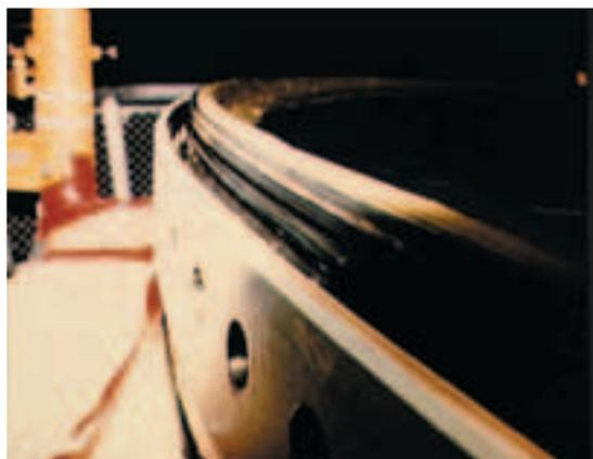
**The booster rocket 'O' ring seal used on the space shuttle**
