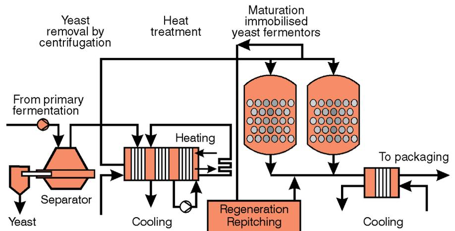
**Figure 4: A two-hour continuous maturation system**
