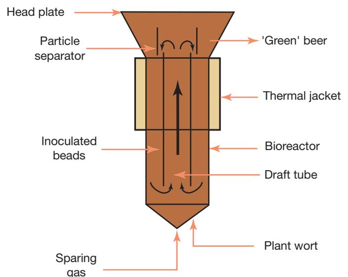
Figure 3: Pilot scale gas lift draft tube bioreactor for primary fermentation of wort
