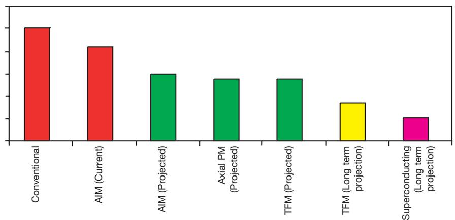
**Figure 8: Comparative size of different propulsion motor technologies**
