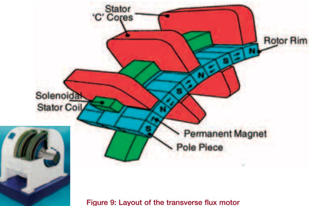
Figure 9: Layout of the transverse flux motor
