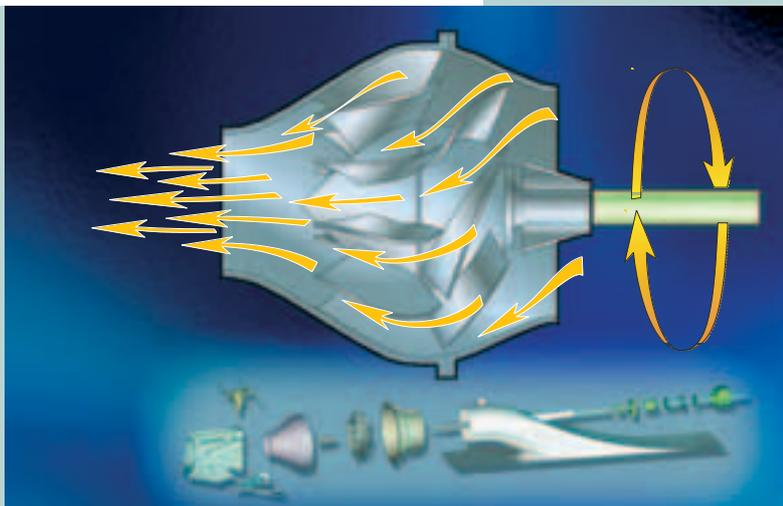
**Figure 5: Construction and water flow through a waterjet**
