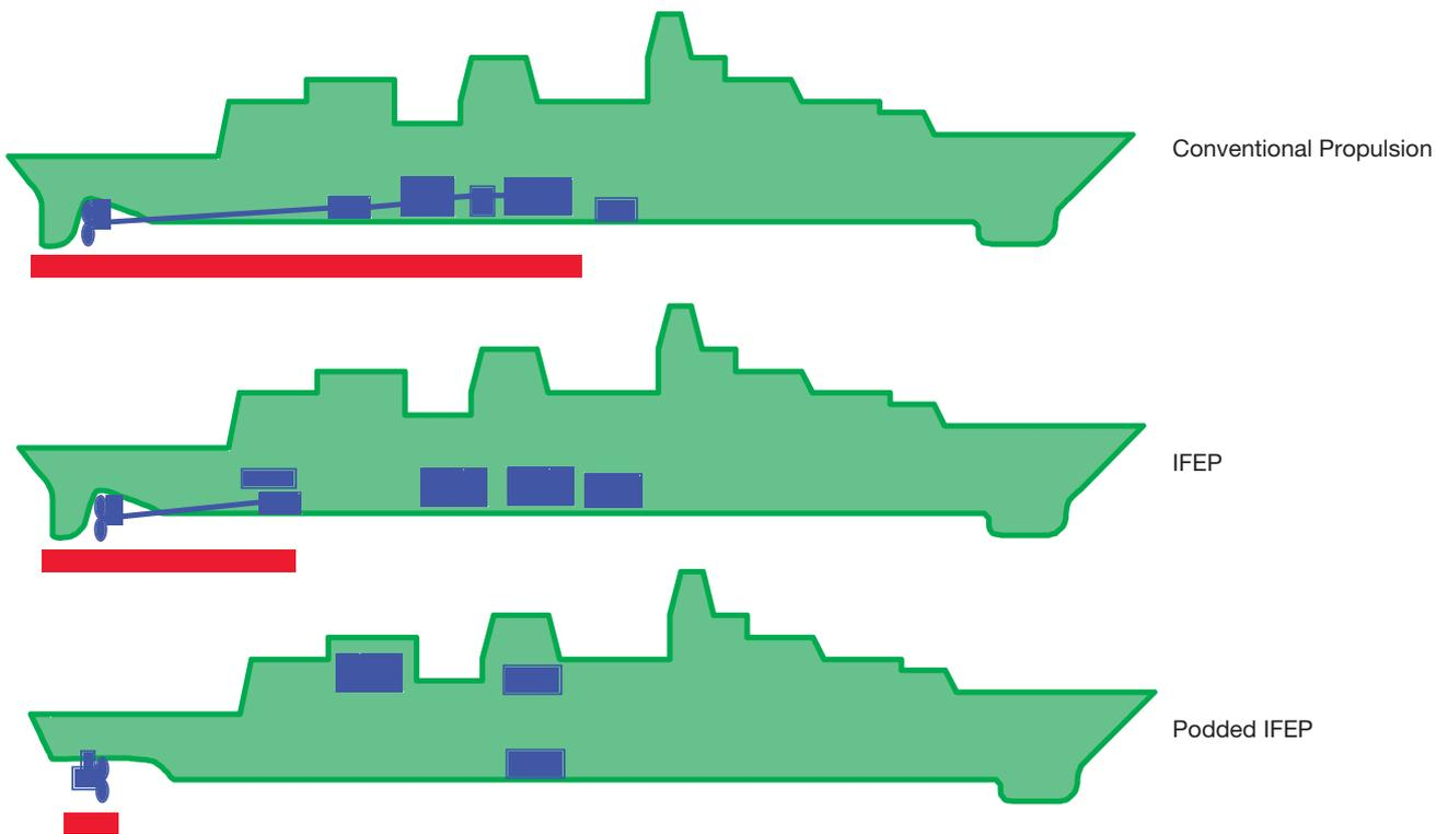
**Figure 7: Layout of mechanical and electrical propulsion systems**
