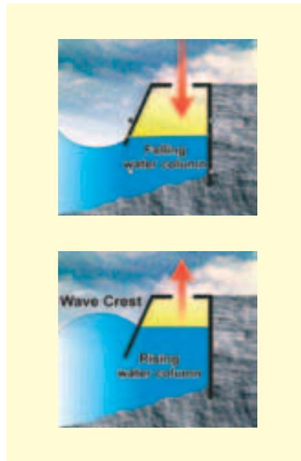
**Figure 4: The principles of operation of an OWC**
