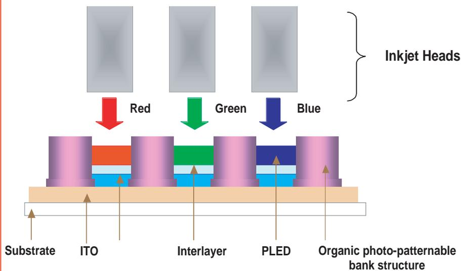
Figure 2 Schematic of the inkjet printing technique for PLED materials
