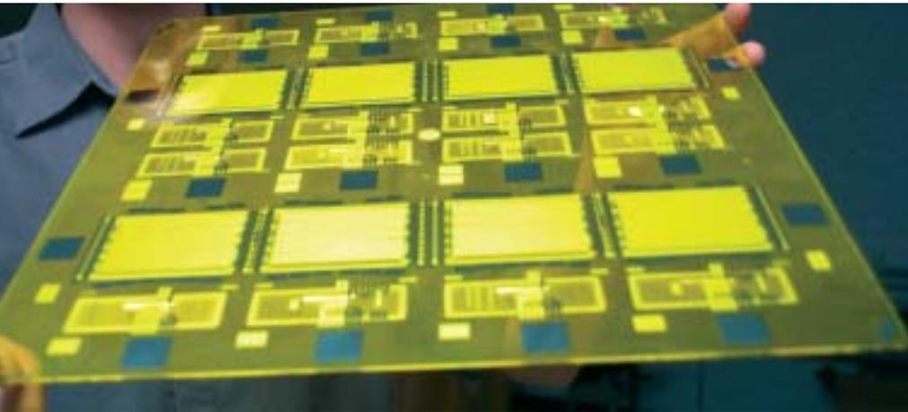
Figure 4 PLED test cells
