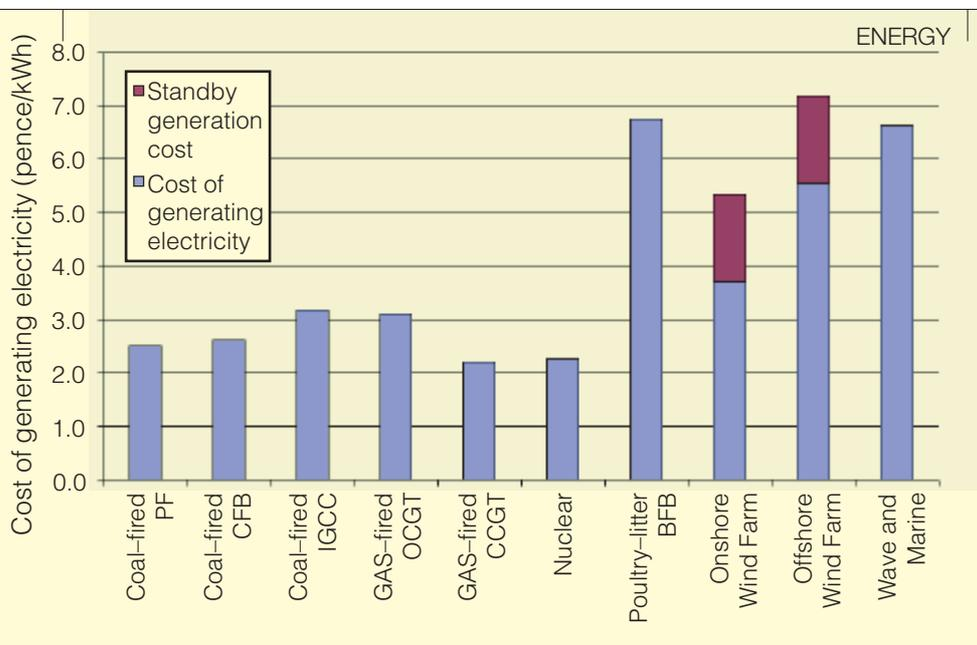
Figure 1 Cost of generating electricity (pence per kWh)
