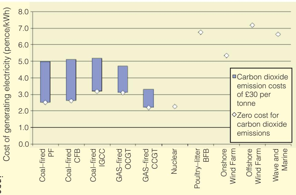
Figure 3 Cost of generating electricity with respect to carbon dioxide emission costs. (£0-30 per tonne)
